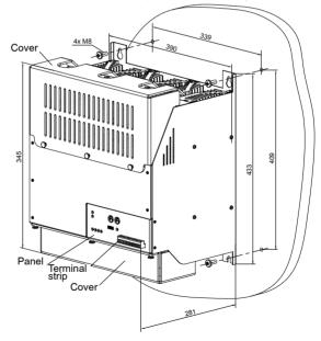
Fig. 4.2.a. Overall dimensions and fixing way of the power controller for 200 A, 300A i 450 A vesions.
