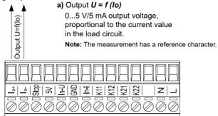
Fig.4.8. Analog outputs.
