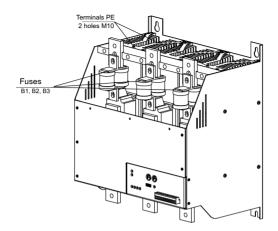
Fig. 4.2.b. he position of the power controller fuses for 200 A, 300A and 450 A versions (view after removing the cover)
