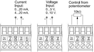
Fig.4.6. Connection of control signals.
