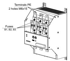
Fig 4.1.b. The position of the power controller fuses for 40 A, 70 A and 125 A versions. (view after removing the cover)
