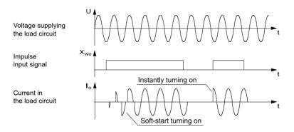
Fig.6.1. Control of on-off type, runs of occurring signals in relation to the neutral wire - resistance load.
