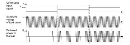
Fig. 6.2. Impulse control with a variable impulse frequency, runs of occurring signals .
